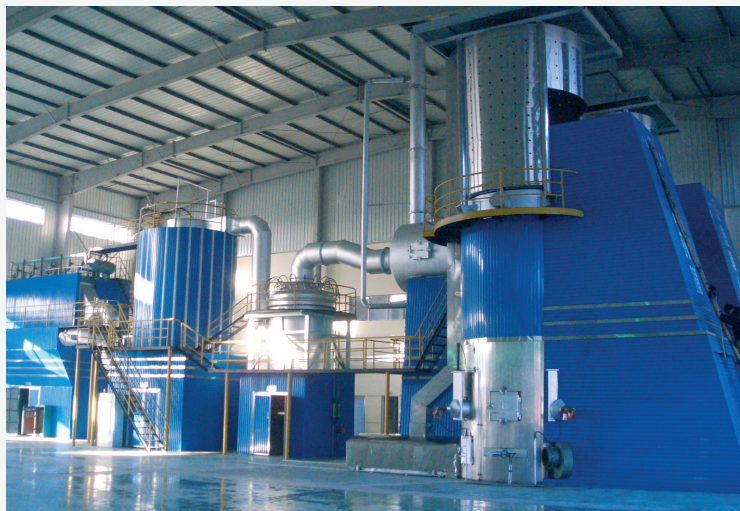
LFY-32 medical waste incinerator with a daily disposal capacity of 32 tons located in Nangong (Beijing)
