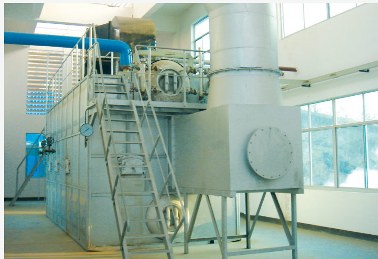
LCH-100 municipal waste incinerator with a daily disposal capacity of 100 tons located in Zhuji
