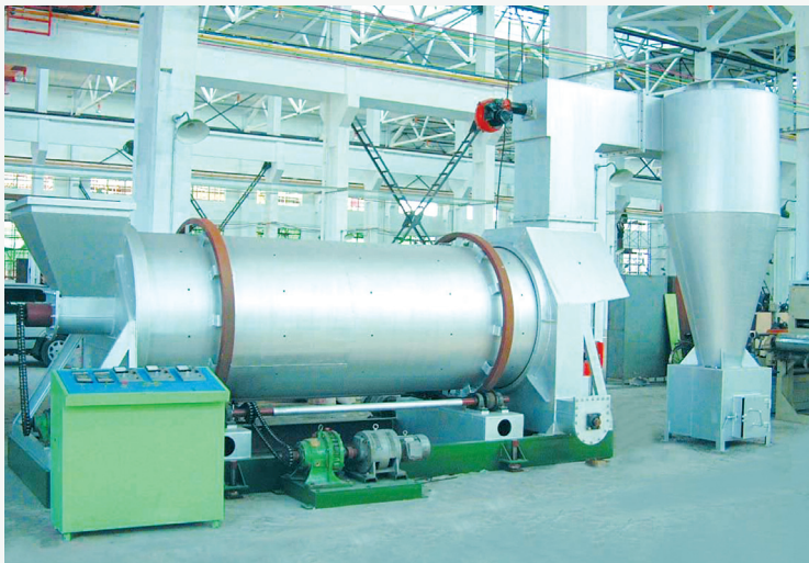
LRX-3 incinerator for industrial hazardous waste with a daily disposal capacity of 3 tons located in Zhuhai
